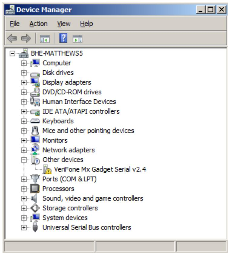
If it is not successful then 'Unrecognised Device' will be displayed instead of 'Verifone Mx Gadget v2.4'. So, if you see 'Unrecognised Device' you know the failure was in the hardware enumeration.
